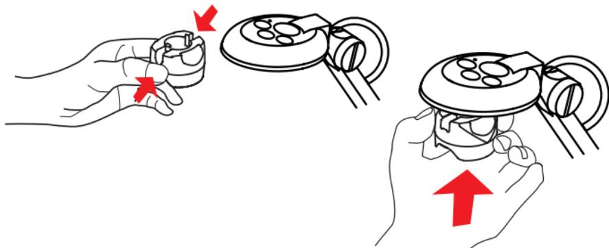
5. Connect the lens with microscope adapter to the microscope.
