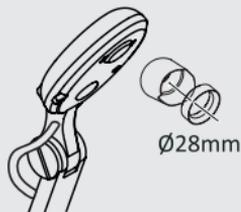
4. Mount / take off the microscope adapter onto / off the lens by doing the action shown in the picture.
