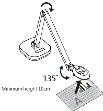
Note : Use two coins to tighten the screws if the arm is loose.
